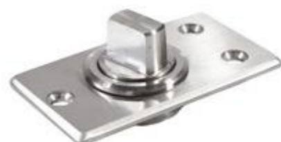
PCA-KZ02 Bottom Pivot 50 kg | Max. Weight Stainless Steel 304 | Material Satin | Finish
