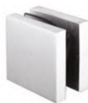
PCA-GC18 Glass - Wall Clamp 25 kg | Max. Weight 10-12mm | Glass Thickness Aluminium | Material Natural Anodize | Finish
