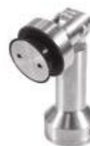
PCA-FC03 Facade Wall - Glass Clamp 10-12mm | Glass Thickness 50 kg | Max. Weight Stainless Steel 304 | Material Satin | Finish
