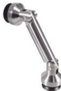
PCA-FC01 Facade Glass - Glass Clamp 10-12mm | Glass Thickness 50 kg | Max. Weight Stainless Steel 304 | Material Satin | Finish
