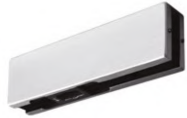
PCA-FH26 Facade Bottom Fitting 10-12mm | Glass Thickness 80 kg | Max. Weight Aluminium, Stainless Steel 304 | Material Natural Anodize, Satin | Finish
