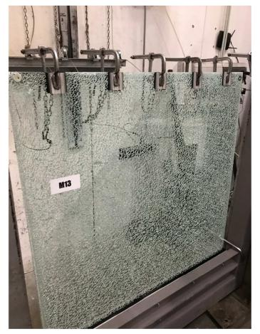
Photograph of the railing after breakage
